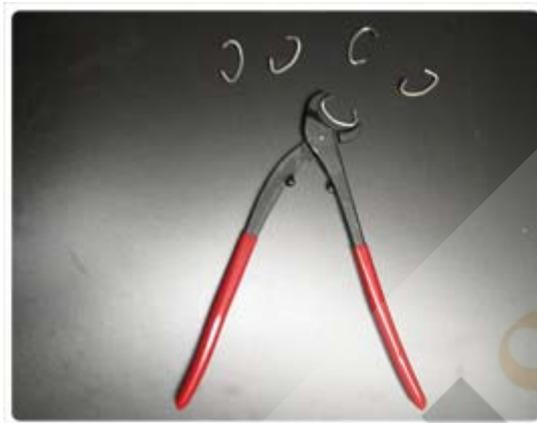
We recommend the c-clamp for fixing razor wire as they are produced solely for this purpose. The c-clamps are made of stainless steel and have a diameter of 3.5mm.
